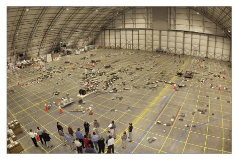
In a hangar at KSC, pieces of debris from Columbia lie across the grid on the floor on 28 February 2003. Members of the Columbia Restoration Project Team examine pieces and reconstruct the orbiter as part of the investigation into the accident. (NASA KSC-03pd0524)
