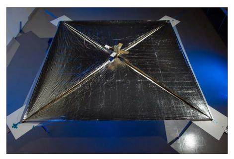
A solar sail, like this one, would use the force of the Sun's photons to propel a spacecraft. This sail is part of a NASA CubeSat called Nanosail-D. (NASA/MSFC/D. Higginbotham)
