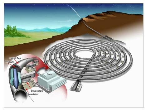
A slingatron from a 22 November 2000 DPT presentation. Slingatrons and blast wave accelerators were potential alternatives to chemical rockets as launch technologies. (NASA from Lisa Guerraelectronic files\Key DPT & Next Briefings\\Exploration Planning.pdf 4/18/05, p. 6)
